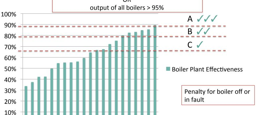
Source: A selection of boilers plants monitored by DCM Logic; each bar represents one boiler plant
